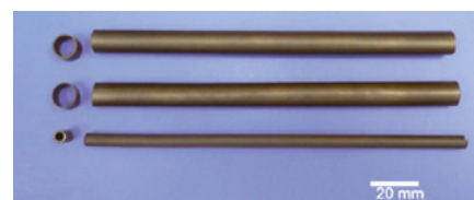
Photo 1 Electroceramics – Oxygen tubular membranes, material: La-Ca-Fe-Co perovskite
