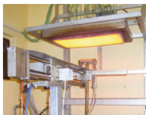
Photo 1 HTC measurement: Continuous casting, secondary cooling
